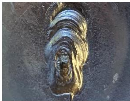
Under Cutting, Too Much Heat Flame is too big and hot for thickness of steel. Puddle is below surface with obvious sunken edges.
