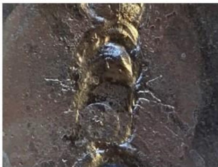
Carburizing Flame Acetylene correct, low oxygen. Obvious secondary cone. Sloppy puddle.
