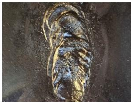
Neutral Flame, Good Weld Correct oxygen-acetylene. Puddle flows into joint, is very still, few sparks, surface tension pulls the joint together.
