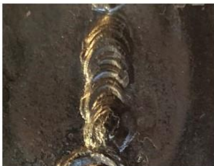
Neutral Flame, Good Weld Correct oxygen-acetylene. Puddle flows into joint, is very still, few sparks, surface tension pulls the joint together.
