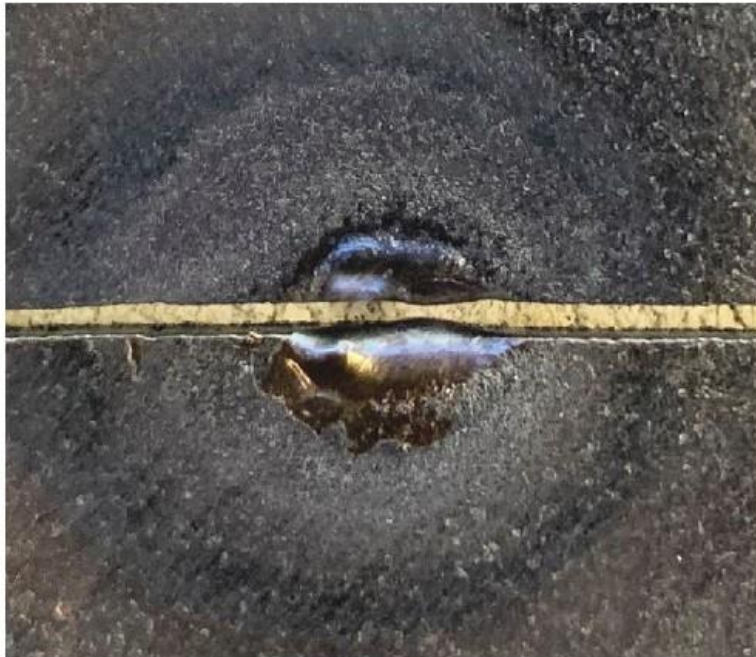
If two edges are present, the corners will melt first and, ideally, surface tension will form the globs into a puddle. FYI- the practice pieces are spaced up from a fire brick by "V"s made of 1/16 welding rod. If there's no space, the brick pulls heat out of the weld.
