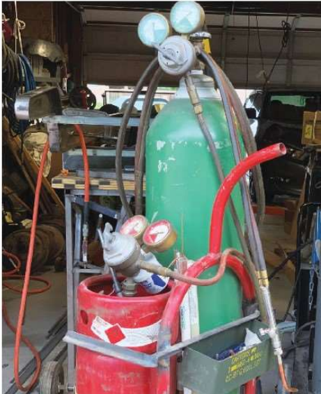
The cheapest dolly, a little angle iron, a .30-caliber ammo can with the top cut off, and a ratchet strap puts you in business. Some practice welding sticks it together. Next time I'll probably go with a .50-caliber can. This unit is 25 years old.
