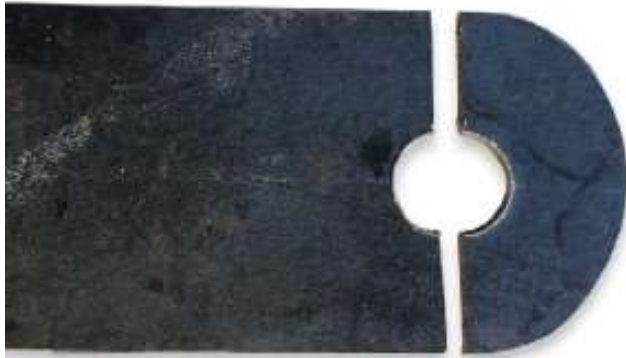
The crosswise failure is due to too much load and not enough steel on that line.
