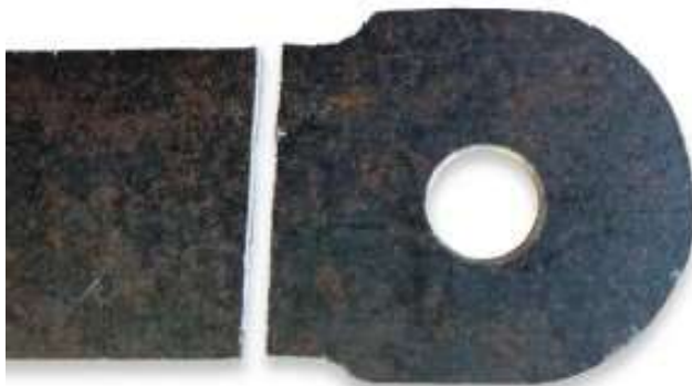
The shank failure is the same as above. Reducing shank width must be done carefully.
