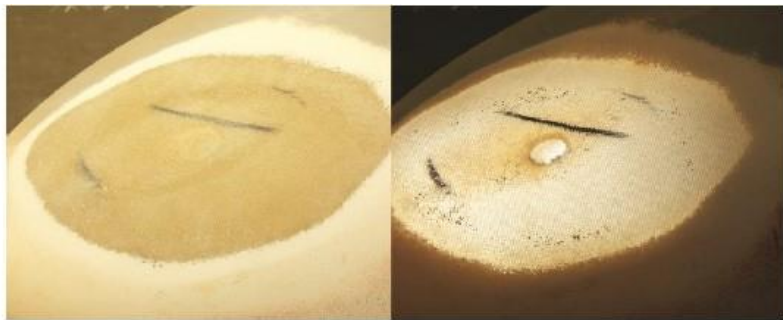
Figure 3: Backlit inspection showing improper scarfing of repair area.
