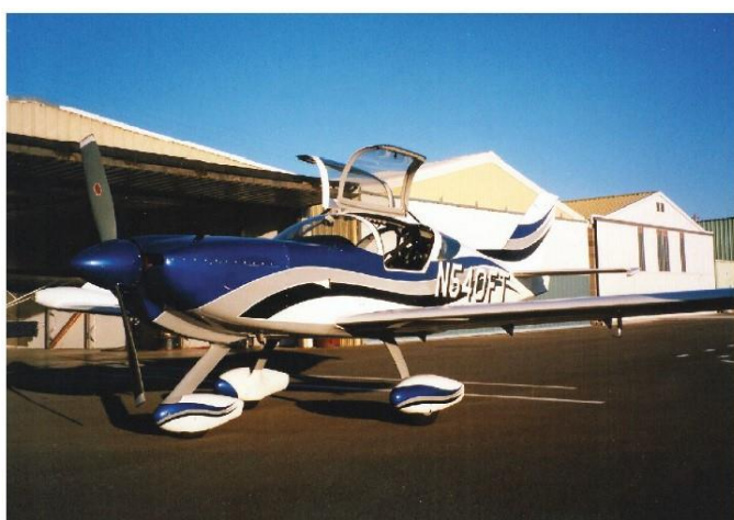
Figure 1: Brian's first composite aircraft project, a Glasair Super II FT with a Lycoming IO-540.
