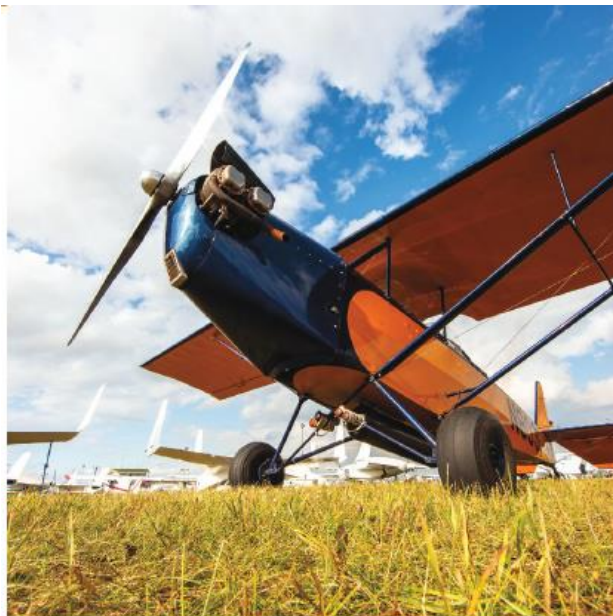
The Pietenpol is a simple and timeless design that has made good use of wood and fabric construction for more than 90 years. The group of Burt Rutan designs in the background shows the incredible depth of homebuilt design and materials use.
