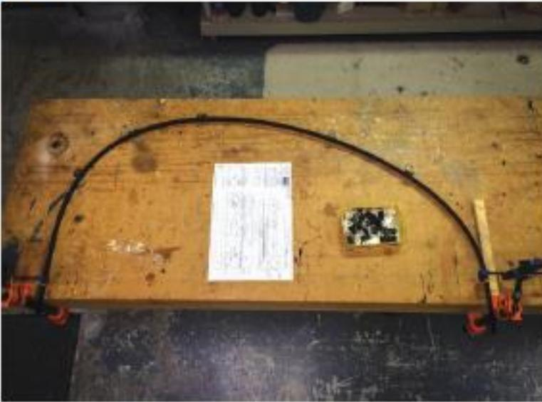
Using the coordinates on the factory drawings, he laid out the curve on his bench and drove 6d finishing nails in around the curve. He then flexed 1-1/4-inch wide steel banding around those nails and clamped it to each nail using big, spring-type paper clips, establishing the curve. The banding came from a lumber yard where it was used for bundling lumber for shipment. He traced that curve on the bench.
