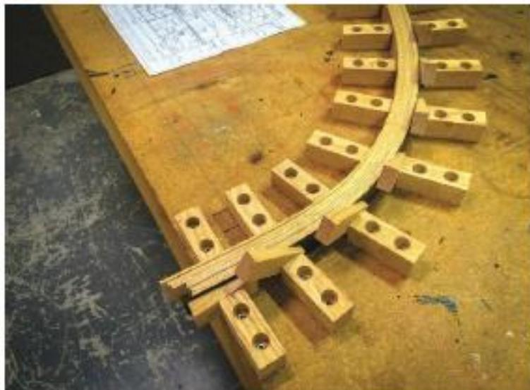
Several dozen blocks were sawed out of oak and positioned around the curve established on the bench. Note that the noses on the inner blocks were slightly curved to allow them to make a single-point contact on the strips. The outer ones are left square, and enough room is left for the healthy wedges shown to be pounded into place. The strips are grouped with no glue and tried in place to make sure all of the spacing is right and that there are no surprises. Literally a "dry run."
