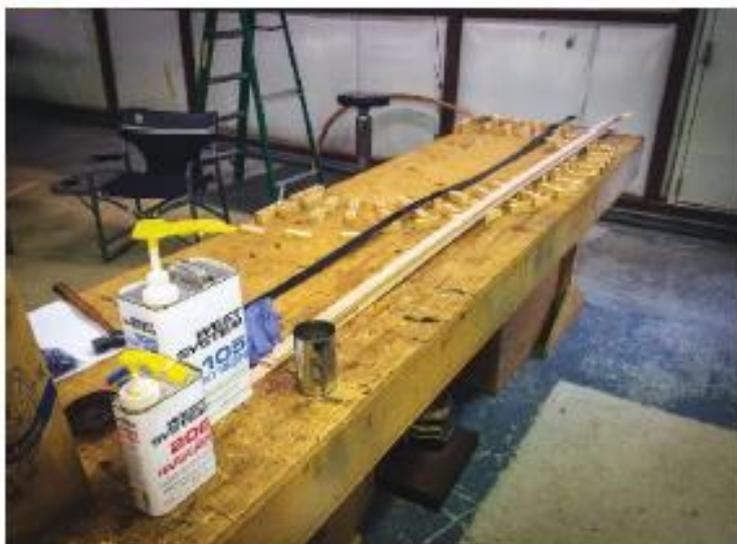
*The makings ready to go. His workbench is built like a hollow-core door, skinned top and bottom, totally true and very stiff. For laminating the tips, he used straight grain, clear mahogany he purchased as 3/4-inch planks. He band-sawed them to 1/8 inch. You can see from their length how big a D4D's wingtips are. The curve is so big that steaming isn't required.*
