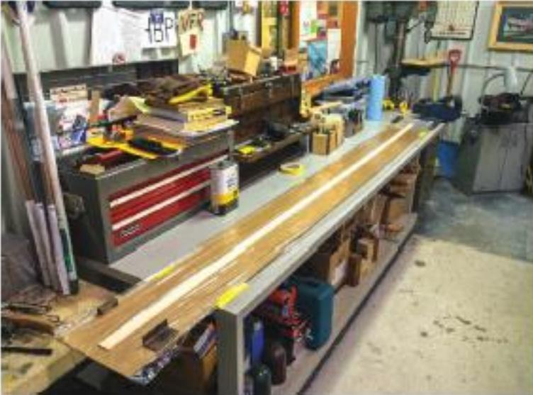
*Plastic wrap is critical to what is a very messy process because the West System epoxy won't stick to it. Each strip is liberally coated with the epoxy on the bench that is protected by plastic wrap. When all of the strips (nine were needed for each tip bow) are liberally coated, they are stacked together on top of a sheet of plastic wrap that is then wrapped tightly around it, forming a tight but squishy bundle.*
