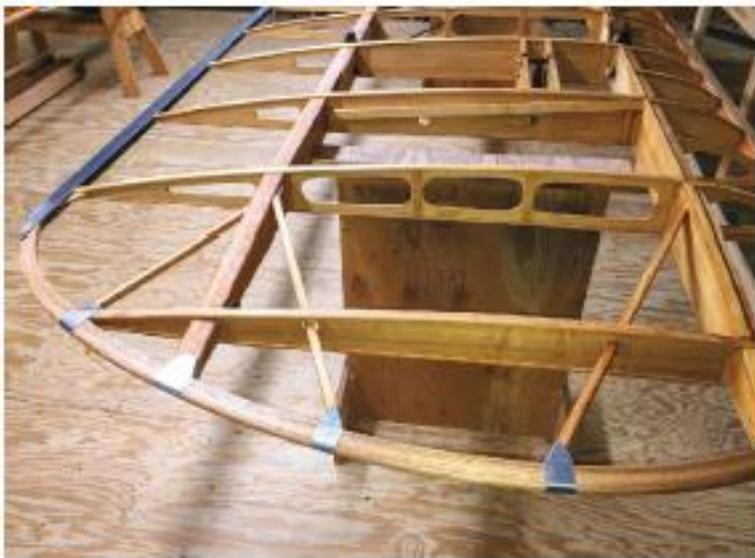
*The finished product! When still in its square, bundled shape, the bow was screwed to the spar tips and shaped with a block plane that Rick said was "very sharp." The sharpness of the plane can't be over-emphasized because the grain in the wood reverses direction every lamination because the strips were alternated in direction for additional strength while laminating. The final shaping was done with sanding blocks.*
