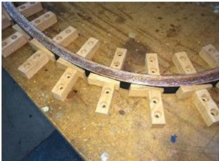
*The bundle is inserted into the blocks with a steel band on both sides. The band spreads the clamping load, making it more even. Then, starting at one end to allow the strips to move slightly and align of their own accord, the wedges are inserted and pounded in until adequate pressure is applied. Left to cure overnight, Rick reports there was only a 2 percent spring-back when the wedges were removed the next morning.*
