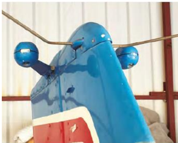
V_{NE} on Piper PA-24s was restricted by an airworthiness directive until a Piper balance weight service kit (pictured here) was installed that placed weight forward of the rudder hinge line.
