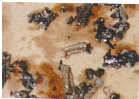
This shrapnel was too big to pass through the suction screen, so was never spotted during oil filter inspections.
