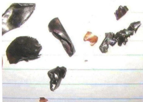
If you rely solely on oil filter inspection and oil analysis, you'll never know about stuff like this. Here's what was left of the Lycoming's flying oil nozzle.
