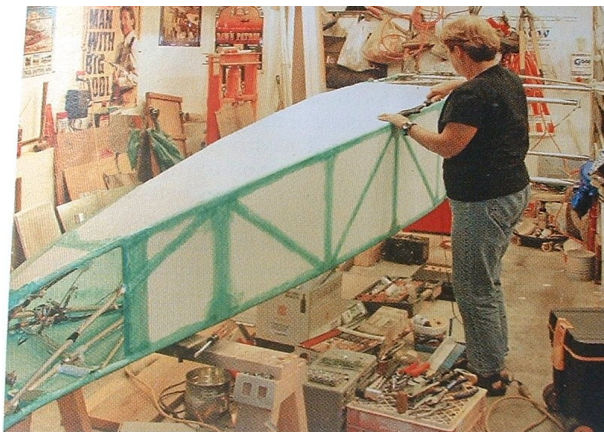
Sharon irons down the edges of the fuselage overlaps in the covering
