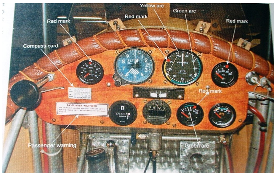
Dick created this illustration to show all of the range and safety marks that had to be in place before the inspection.
