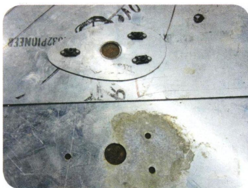
Corrosion rears its ugly head under the doubler plate.
