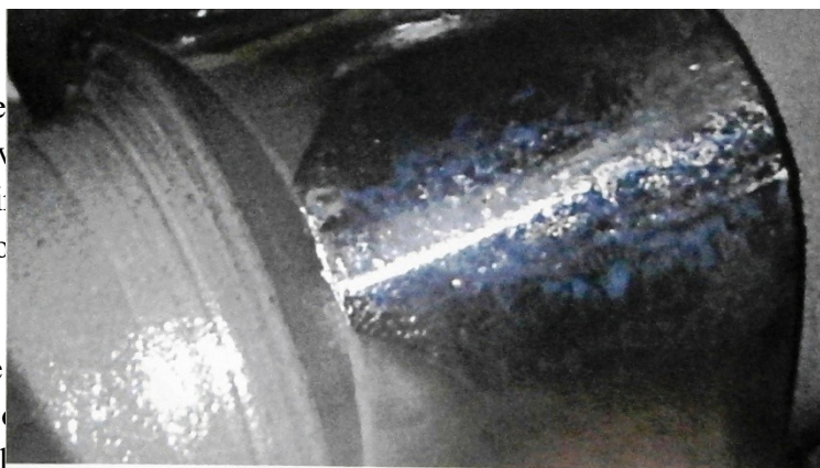
Figure 3—This close-up of the questionable cam lobe suggested that the distress is still minor and the engine could remain in service with 100-hour lifter inspections.
