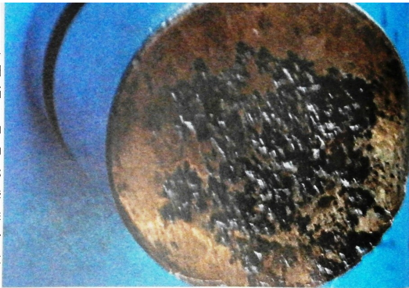
Figure 2—This lifter is severely spalled and clearly unairworthy. But on big-bore Continental engines, lifters are cheap and easy to replace.
