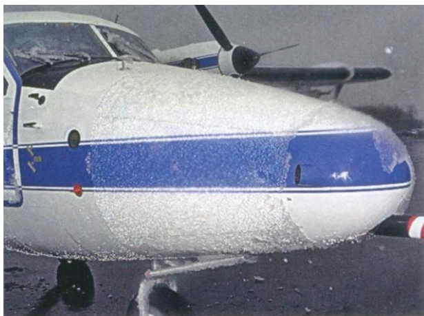
Ice contamination as a result of encountering supercooled large droplet (SLD)
