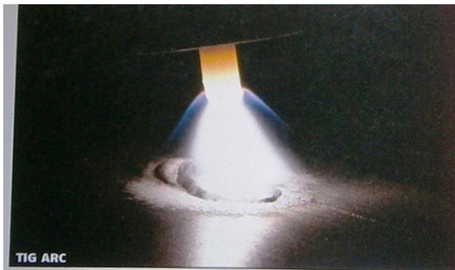
*The arc is struck between the work surface and the tungsten electrode. As the heat is increased, the surface is melted and a puddle formed. Rod is momentarily fed in, then withdrawn, which forms the "stack of dimes" bead.*
