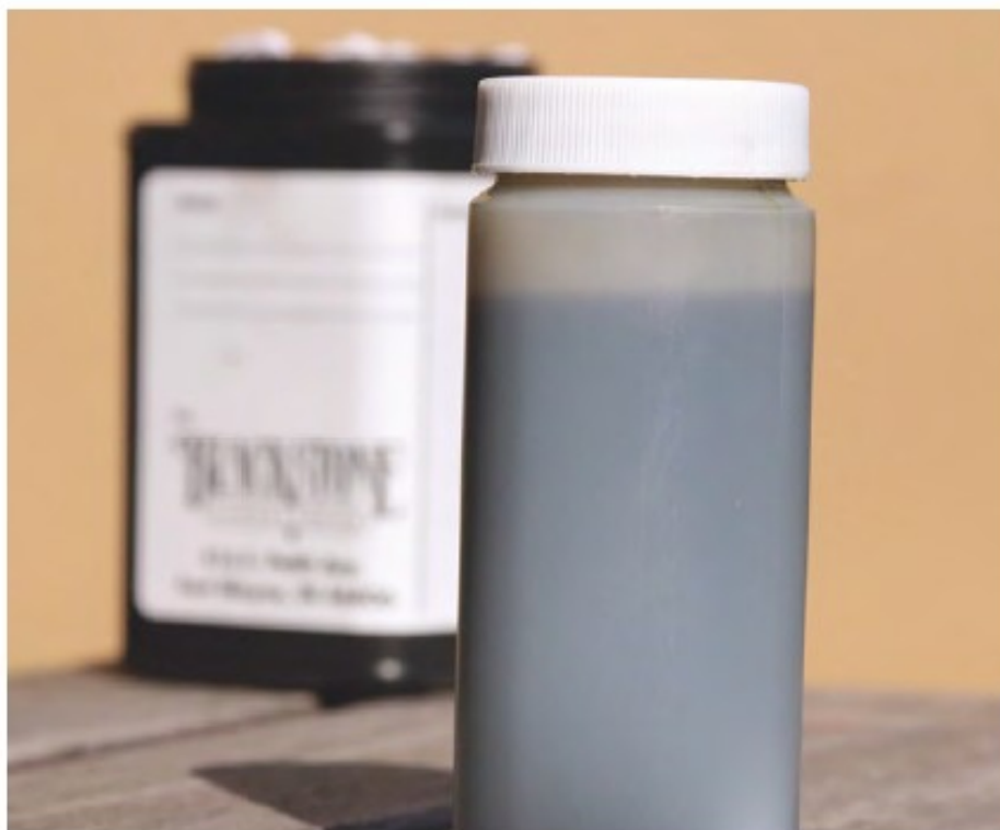
Above: A series of oil samples are required to establish the wear baseline for an engine.
