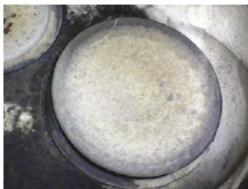
Right: A borescope is essential in determining cylinder health. This is the No. 4 exhaust valve in my Lycoming O-360 engine.
