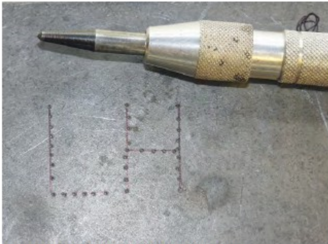
Mechanical punch used to ID tooling, etc. Not to be used on airframe parts.
