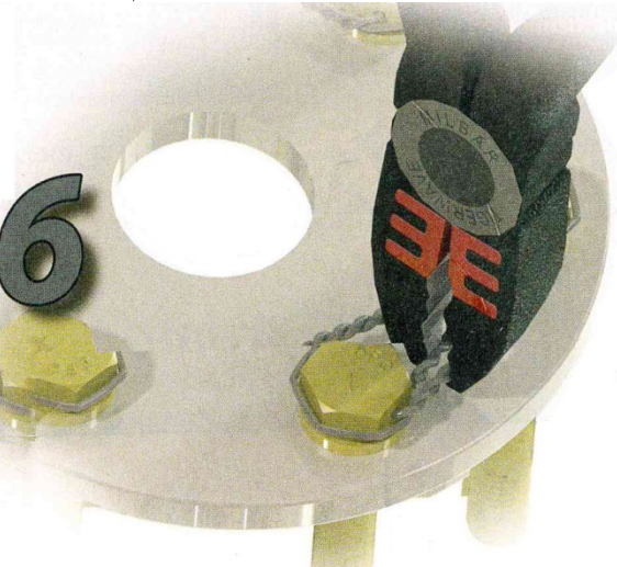
Figure 6: Double-twist safety wire procedures.
