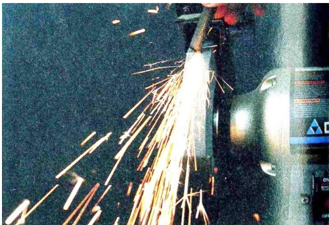
Figure 1: Spark Testing Ferrous Metals With a Bench Grinder
