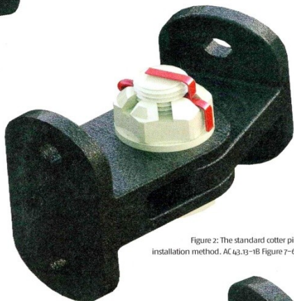
Figure 1: The tuck method for installation of cotter pins. Note: Cotter pins shown in red for vivification.
