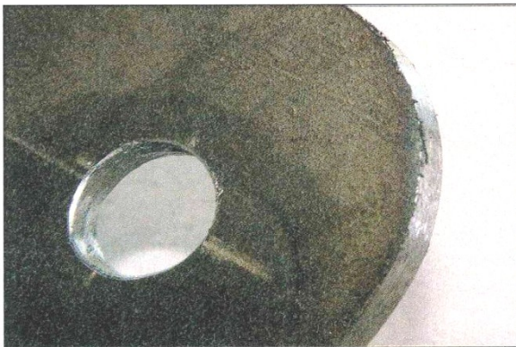
Final sanding should always follow the edge. However, the 150 grit still leaves sharp edges and lots of scratches.
