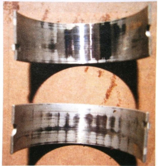
Figure 13—This bearing exhibits severe overload damage, probably due to detonation or preignition.
