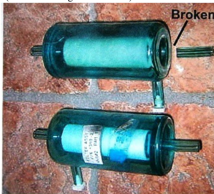
Figure 3—Fracture of this plastic magneto pressurization filter caused simultaneous and severe high-altitude misfire of both magnetos. So much for redundancy..
