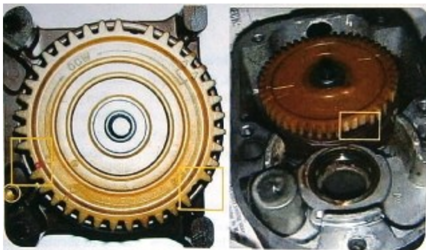
Figure 1—Distributor gear failures like these can cause a magneto to start firing random spark plugs at random times.
