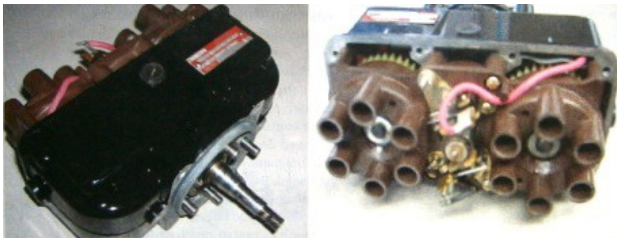
Figure 2—The Bendix D2000/D3000 dual mag is basically two independent magnetos packaged into a single unit.
