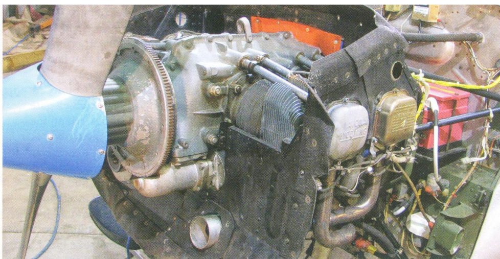
A hole the size of a quarter in engine baffling can raise operating temperature by as much as 20 degrees Fahrenheit.
