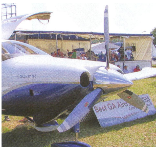
High performance cowling must be matched with appropriate propeller and spinner design for sufficient engine cooling.
