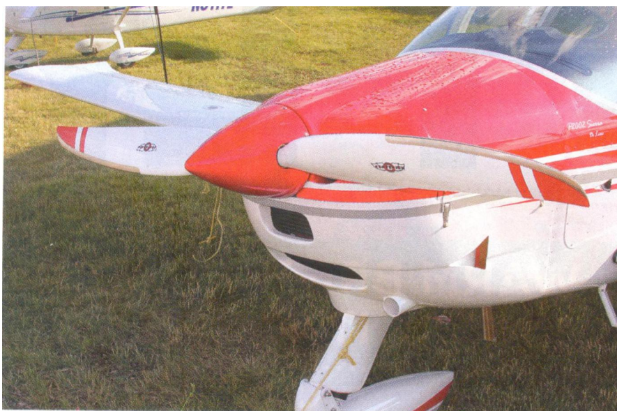
Modern aircraft cowling design provides for reduced drag and efficient engine cooling.
