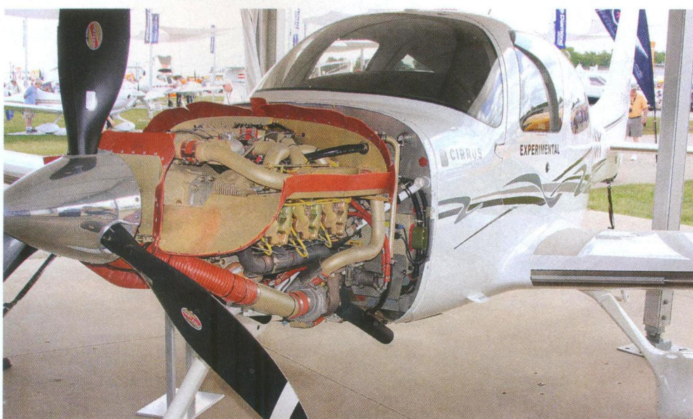
With their high operating temperatures, turbochargers often require direct cooling via flexible tubing.
